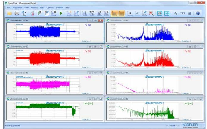
With Kistler DynoWare, up to 16 LabAmp channels can be configured, synchronously recorded and analyzed.
