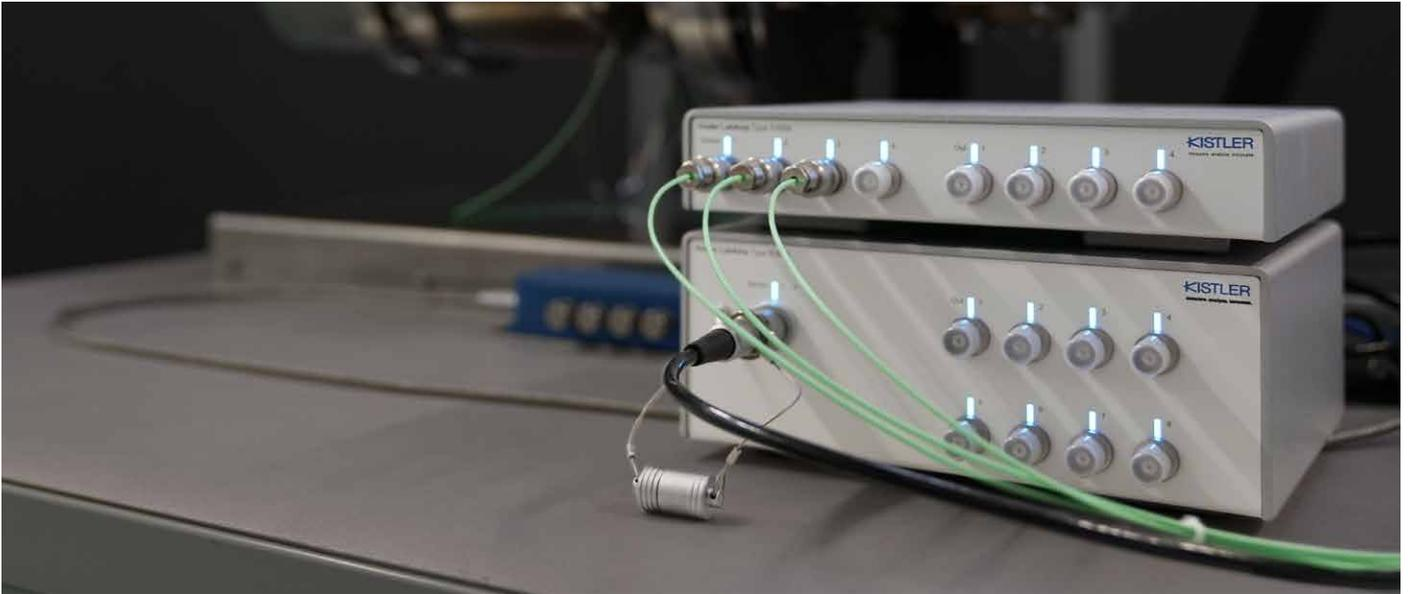
Example rocket propulsion test bench: PTP synchronized LabAmp Types 5167A and 5165A for 6-component force measurement and three pressure pulsation measurements to look for combustion instabilities in the combustion chamber
