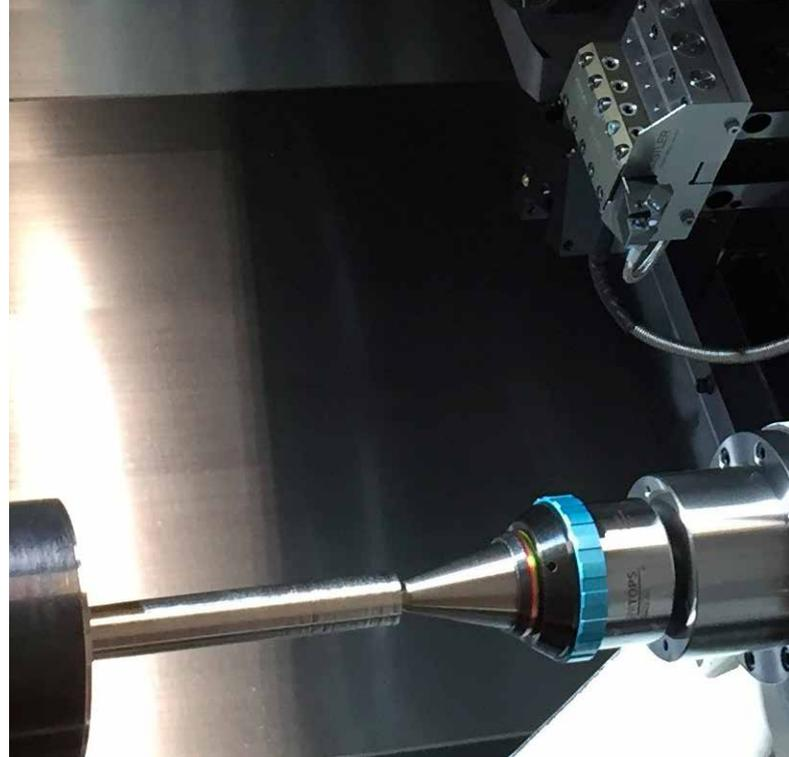
Integration of Kistler dynamometer Type 9129AA in a lathe for machining tests
