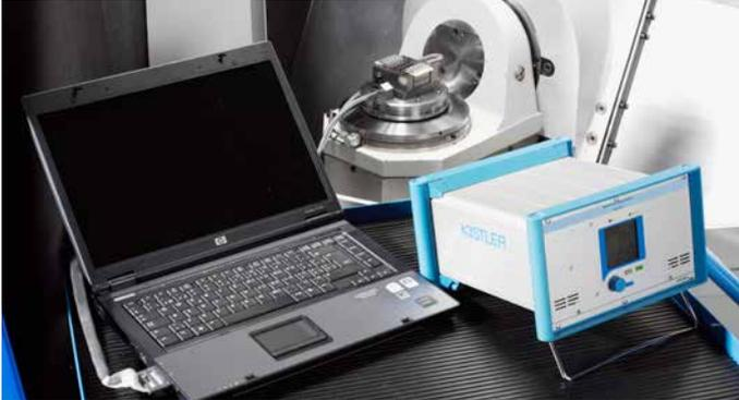
Measurement setup in front of machining center
