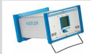
Multichannel charge amplifier 5070A... for multicomponent Force Measurement.
