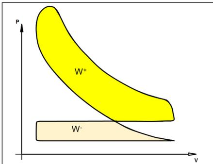
Figure 2: Breakdown of work in terms of thermodynamics into work that can be gained or that must be performed, with the pV intersection point method
