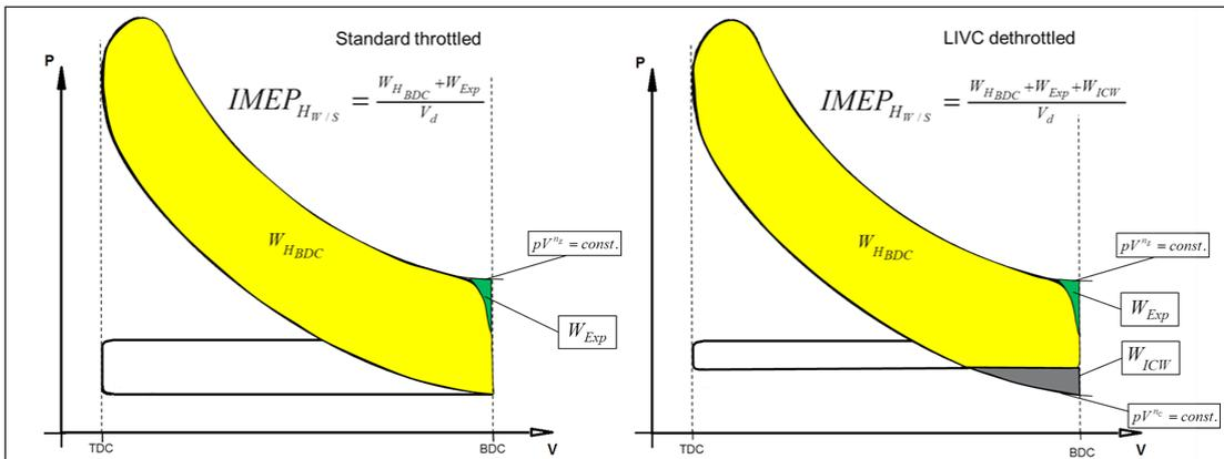
Figure 4: High pressure portion according to Witt/Shelby for the standard process, and with late intake valve close
