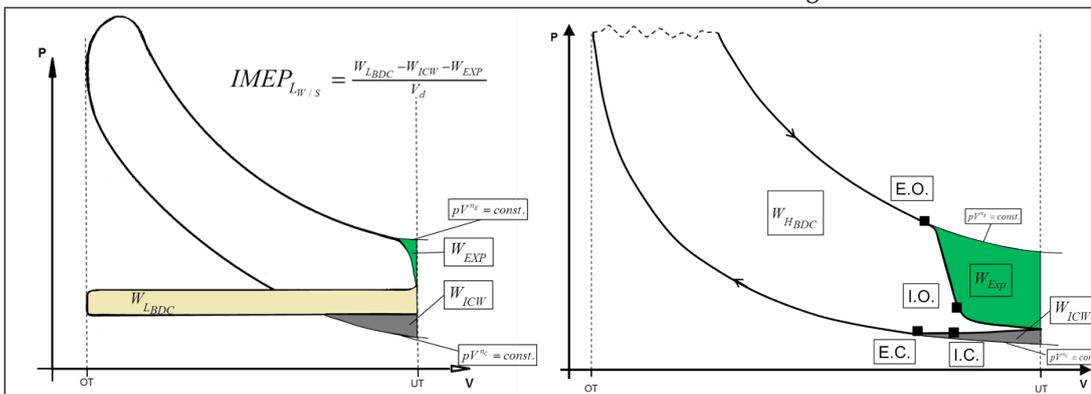
Figure 5: Gas exchange portion according to Witt/Shelby in case of late intake valve close and evaluation of the 2-stroke process
