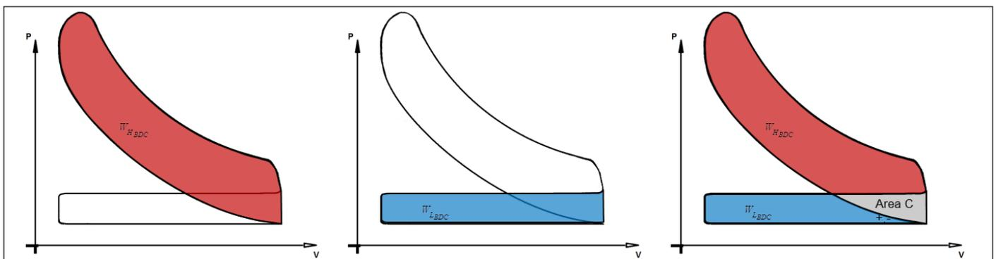
Figure 1: High pressure work, gas exchange work and total work including Area C with the BDC-BDC method (from left to right)
