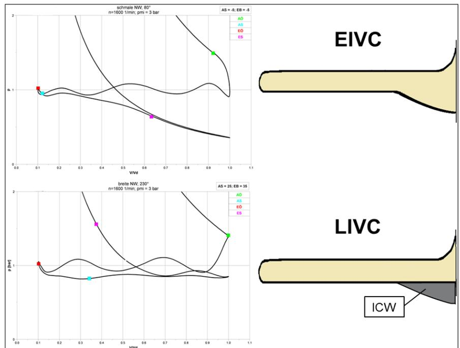
Figure 7: Dethrottling due to early intake valve close (EIVC) and late intake valve close (LIVC)
