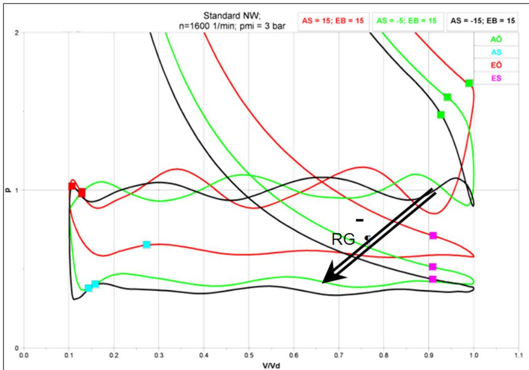
Figure 6: Dethrottling due to residual gas variation over exhaust camshaft phasing
