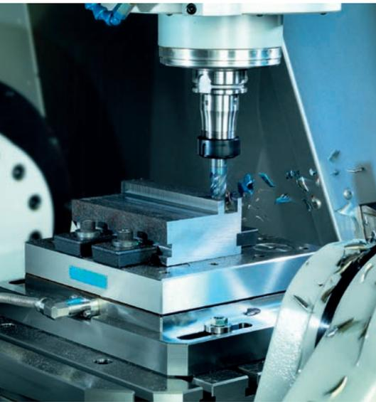
4 Measurement of force while milling with a stationary Type 9255C dynamometer © Kistler
