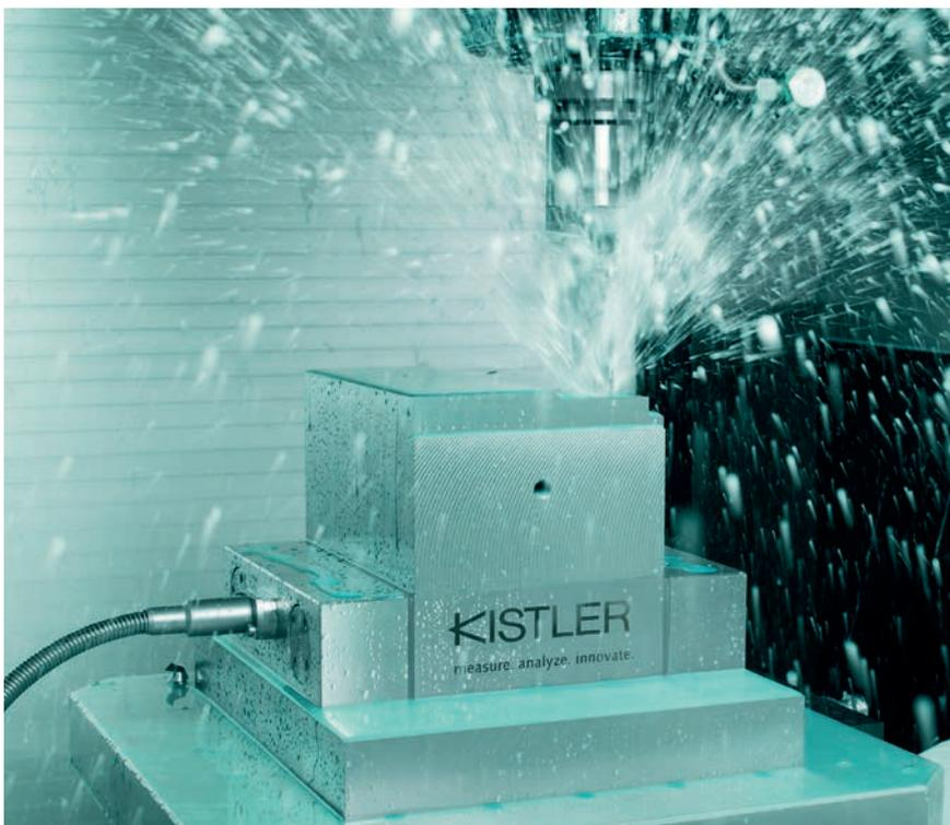
**1** Measurement of the force used in the process permits conclusions about the quality of the surface, wear and general characteristics of materials (© Kistler)
