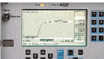
Electrode force is measured during welding and displayed on Type 5857A... control monitor.
