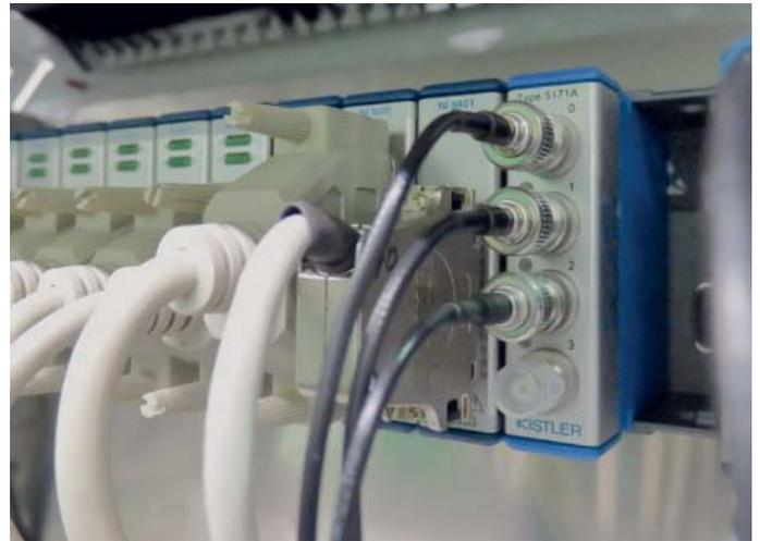
The charge amplifier module Kistler Type 5171A for CompactRIO™ in use
