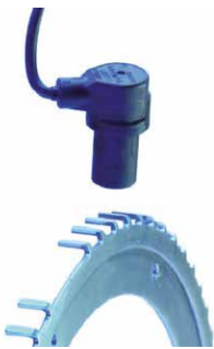
Fig. 10: Processing of the engine's stock crankshaft position sensor
