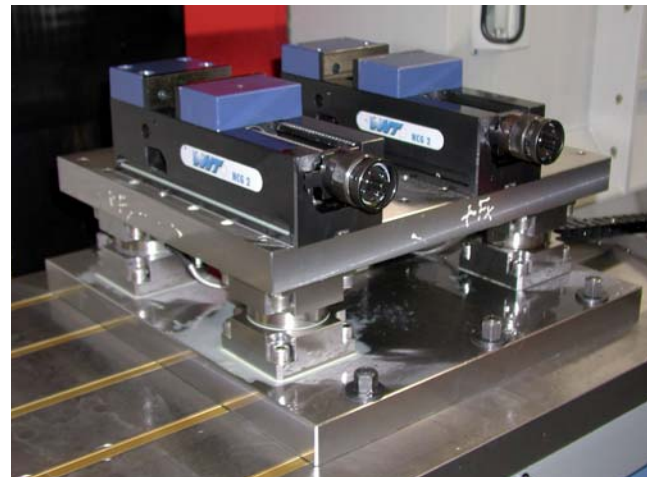
Fig. 1: Cutting force dynamometer constructed with four 3-component force links
