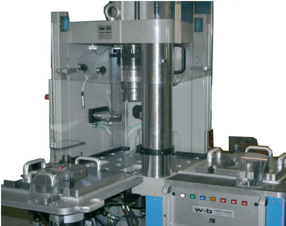
Fig. 6: Movable 3-component calibration unit for full scale recalibration (100 %FSO) of SmartCrash® force measuring elements on customer's site
