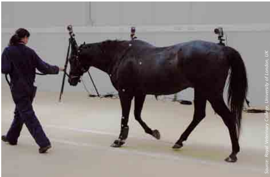
Analysis of the gait of horses on six force plates Type 9287BA installed on the ground
