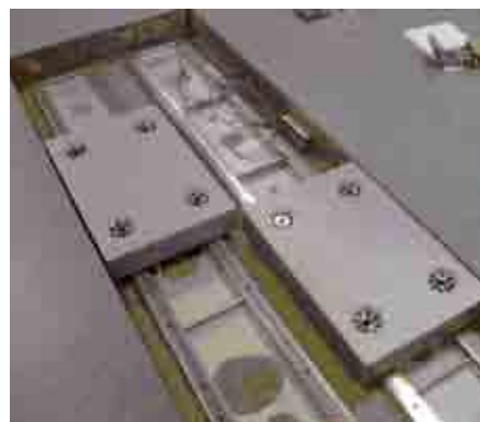
Easy installation and versatility: Two force plates Type 9281EA on frame with variable mounting positions
