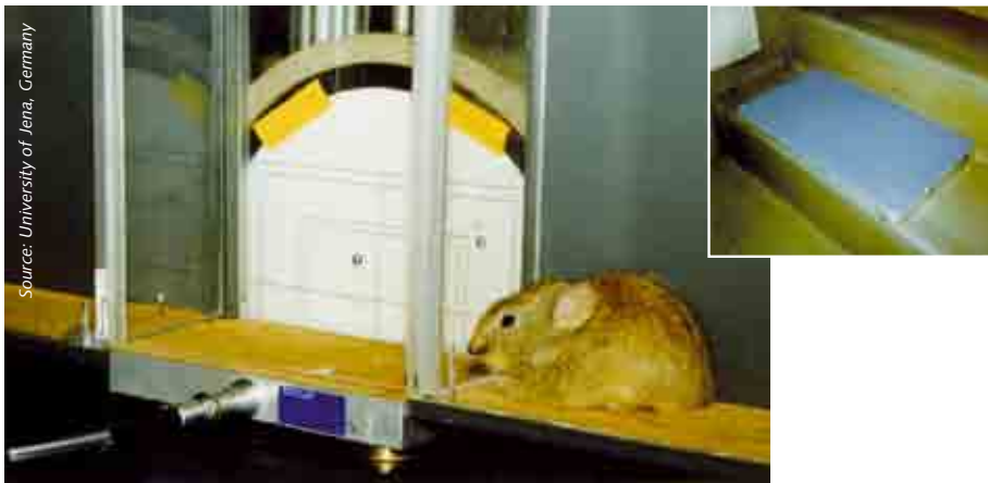
Special-sized force plates, e.g. for stairs (270x500x35 mm, top right) or for experiments with small animals (120x200x35 mm, top), are developed to customer requirements
