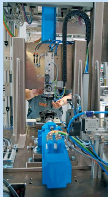
Assembly with NC joining modules in factory of special machinery manufacturer SITEC
