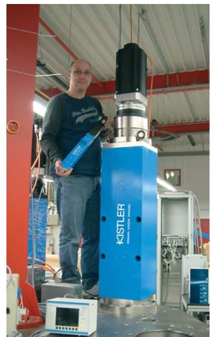
Martin Werner, Service Manager of NC Joining Systems, shown presenting the smallest and the largest Kistler servo press (NCF: 0,5 kN / 1 kN and NCFN: 300 kN)
