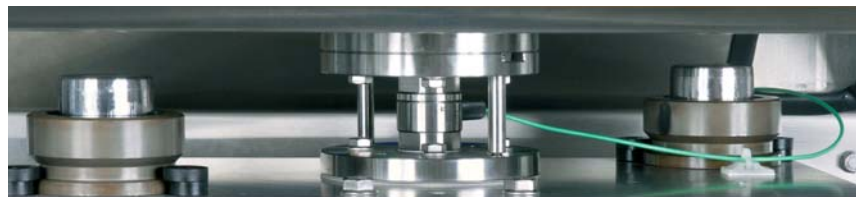
Force sensor Type 9333A in special device employed by manufacturer of filling and sealing systems to determine process parameters for fully automated heat-sealing of packs
